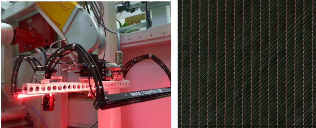
Figure 8: a) Quality assurance unit (OCQU); located on the left, on the 6-axis articulated-arm robot for recording textile surface defects after deposition; right: examples of an imaged textile surface of a multiaxial carbon fabric with the evaluated fiber orientations (red: sewing threads; green: gaps)
