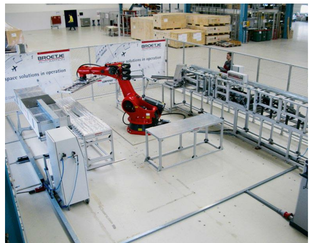
Figure 1 Composite preforming cell (© Broetje-Automation)
