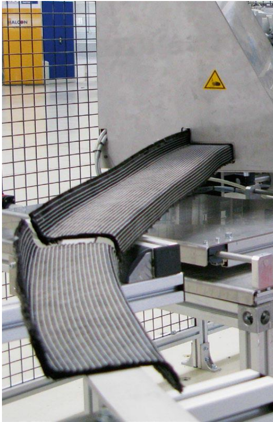
Figure 3 Preforms continuously manufactured with the Continuous Composite Preforming System (© Broetje-Automation)
