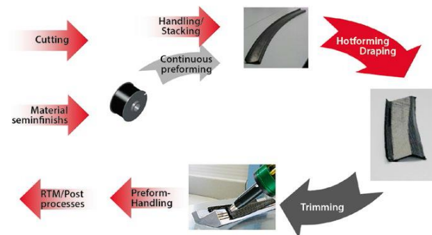
Figure 2 Production process within the Composite Preforming Cell (© Broetje-Automation)
