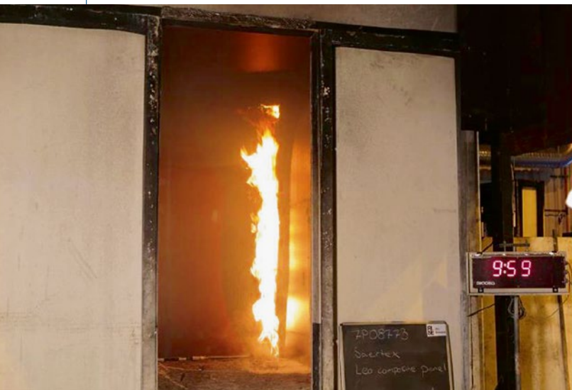
FIGURE 7 Room corner test after approximately 10 min exposure to flame at 100 kW (© Saertex)
