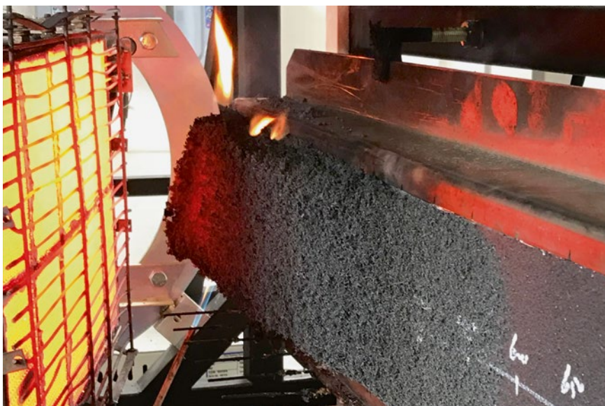
FIGURE 2 Test specimen in the fire safety test in accordance with IMO, Part 5, for measuring flame propagation (© Saertex)
