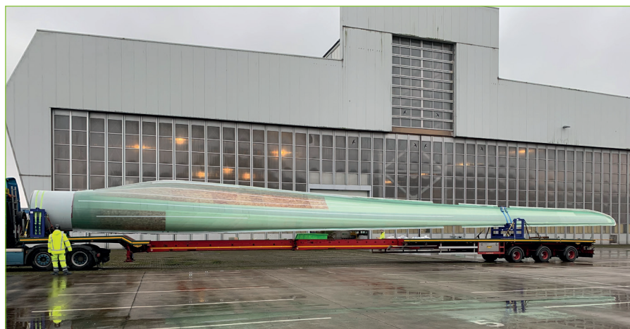
Fig. 1: The sandwich areas made of balsa and PET foam can be seen on an unpainted blade blank
