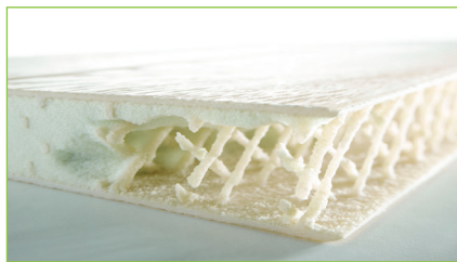
Fig. 2: Reinforced foam core with the foam partially removed to show the internal structure
